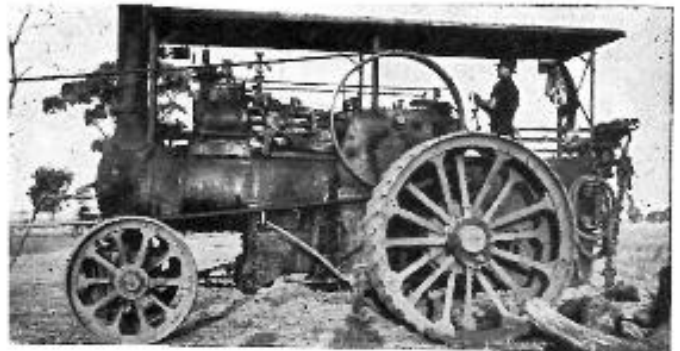
ABOVE: An old Marshall compound steam traction engine at work on "Glenross". The winding drum can be seen on the back driving wheel (February, 1937).
